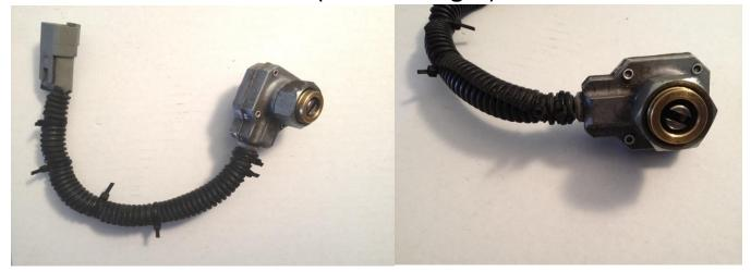
The Speedometer shop creates the unit by melding several components together with an adapter collar and Slotted pin with
